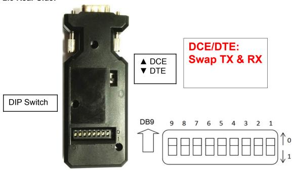
2.4 Default: All pin is "0", Baud rate 9,600 bps., 8 Data bits, None parity, 1 Stop bit.
